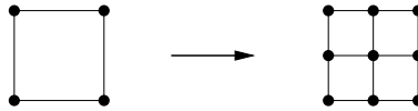
FIGURE 2. The operation of splitting a square face into four smaller square faces.
