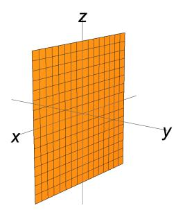
T(x, y, z) = (x, 0, z), so *T* fixes every vector in the *xz*-plane and destroys every vector of the form (0, a, 0) with *a* real. Therefore,  $\lambda = 1$  and  $\lambda = 0$  are eigenvalues and in fact they are the only eigenvalues since their combined eigenvectors span all of  $\mathbf{R}^3$ .
