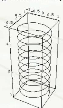
Helix  $F(t) = \cos(4\pi t)i + \sin(4\pi t)j + tk$ Velocity ~ (t) = -4TTSIN(4At) 7 + 4TTCOS(4TTt) J + k  $specal = \sqrt{(4\pi sin(4\pi t))^2 + (4\pi cos(4\pi c))^2 +$  $=\sqrt{1+16\pi^2}$ Velocity changes, as a vector speed does not change. This is a special fact, USually speed does change
