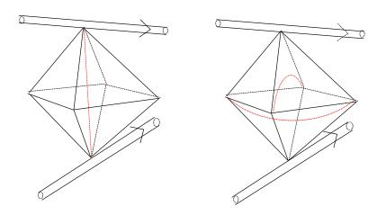
FIGURE 3. Any octahedron can be split into 4 or 5 tetrahedra by adding the red dashed edges to it.
