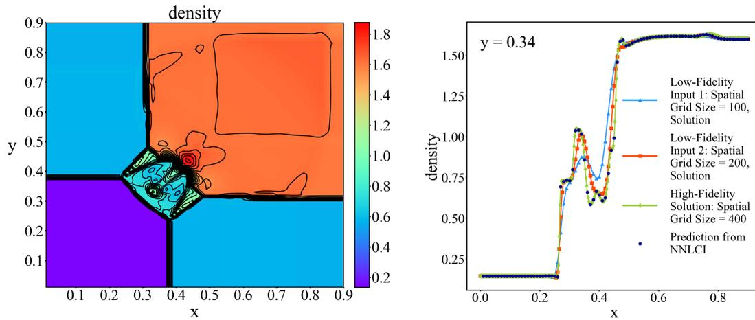
Figure 16: NNLCI prediction of final-time ( $t = 0.3$ ) density distribution of 2D Euler system with initial value +5% perturbed from that of Case 3 (see Table 1), and axial distribution of density (dark blue) along  $y = 0.34$ , compared to low-fidelity input solutions (blue and red) on  $100 \times 100$  and  $200 \times 200$  grids, respectively, and reference solution (green).
