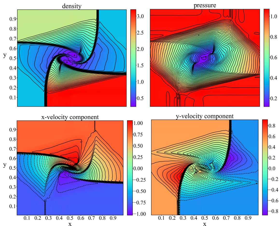
Figure 6: NNLCI prediction of the final-time ( $t=0.3$ ) solution of the 2D Euler system, with initial value +5% perturbed from that of Case 6: density, pressure,  $x$ -velocity, and  $y$ -velocity.
