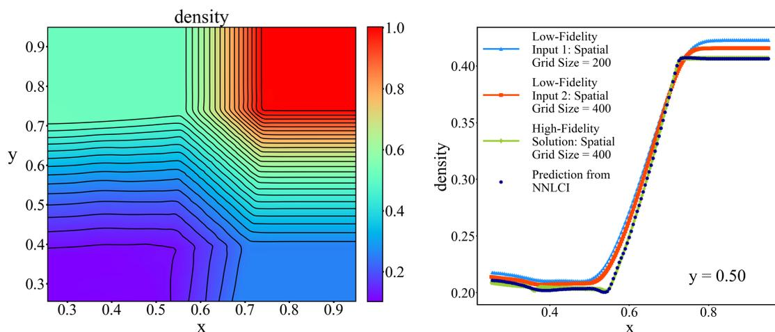
Figure 9: NNLCI prediction of final-time ( $t=0.2$ ) density distribution of Case 1 (see Table 1), and axial distribution of density (dark blue) along  $y=0.50$ , compared to low-fidelity input solutions (blue and red) on  $200 \times 200$  and  $400 \times 400$  grids, respectively, and reference solution (green).
