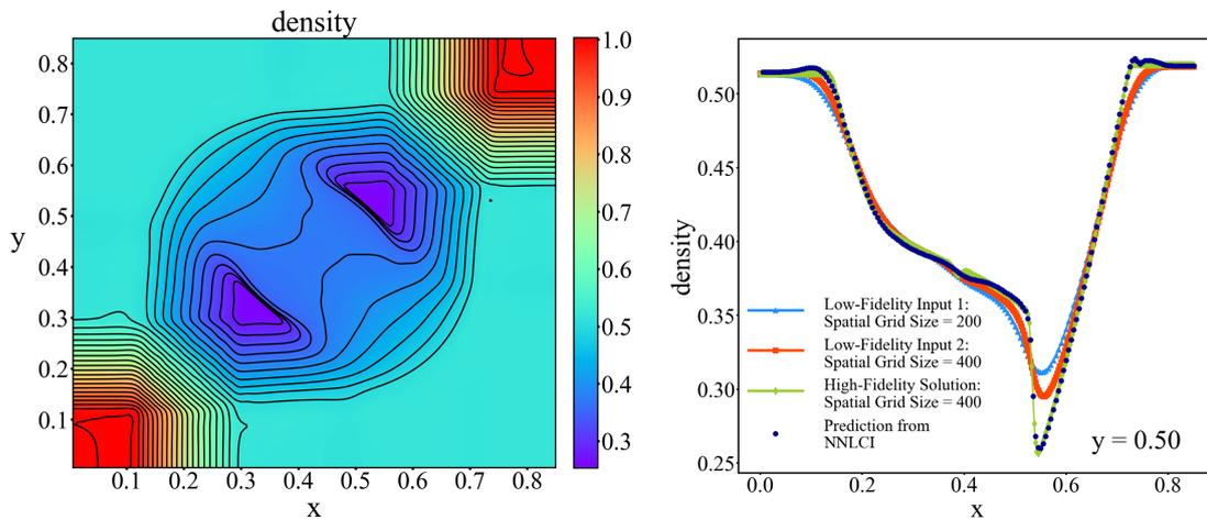
Figure 11: NNLCI prediction of final-time ( $t=0.2$ ) density distribution of Case 2 (see Table 1), and axial distribution of density (dark blue) along  $y=0.50$ , compared to low-fidelity input solutions (blue and red) on  $200 \times 200$  and  $400 \times 400$  grids, respectively, and reference solution (green).
