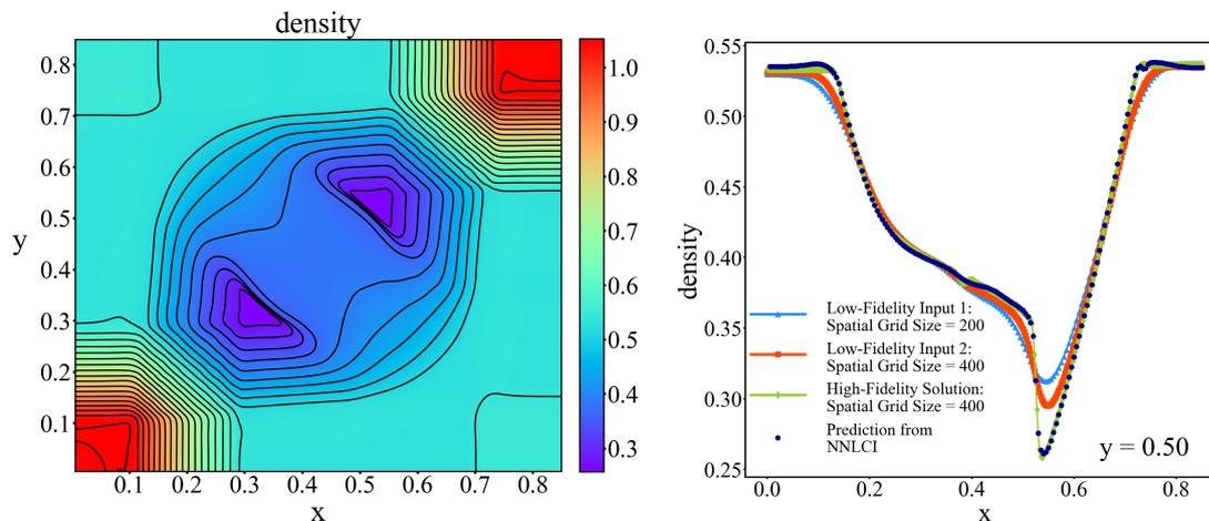
Figure 12: NNLCI prediction of final-time ( $t=0.2$ ) density distribution of 2D Euler system with initial value perturbed by +5% from that of Case 2 (see Table 1), and axial distribution of density (dark blue) along  $y=0.50$ , compared to low-fidelity input solutions (blue and red) on  $200 \times 200$  and  $400 \times 400$  grids, respectively, and reference solution (green).
