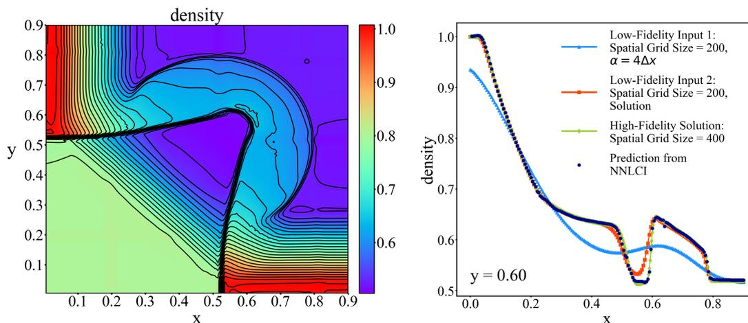
Figure 23: NNLCI prediction of final-time ( $t = 0.25$ ) density distribution of Case 8 (see Table 1), and axial distribution of density (dark blue) along  $y = 0.60$ , compared to low-fidelity input solutions (blue and red) from leapfrog and diffusion splitting scheme (2.9) ( $\alpha = 4\Delta x$ ) on  $400 \times 400$  grid and 4th-order scheme on  $200 \times 200$  grid, respectively, and reference solution (green).
