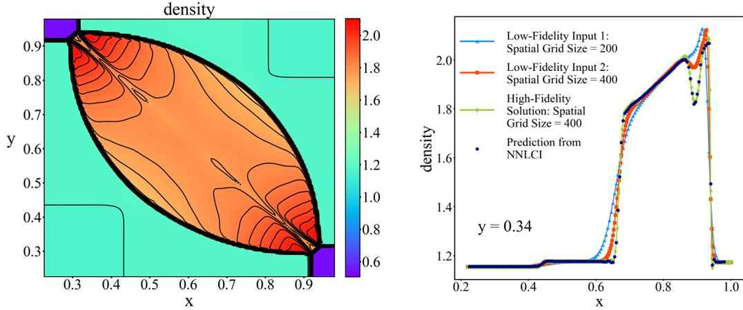
Figure 18: NNLCI prediction of final-time ( $t=0.25$ ) density distribution of 2d Euler system with initial value +5% perturbed from that of Case 4 (see Table 1), and axial distribution of density (dark blue) along  $y=0.34$ , compared to low-fidelity input solutions (blue and red) on  $200 \times 200$  and  $400 \times 400$  grids, respectively, and reference solution (green).
