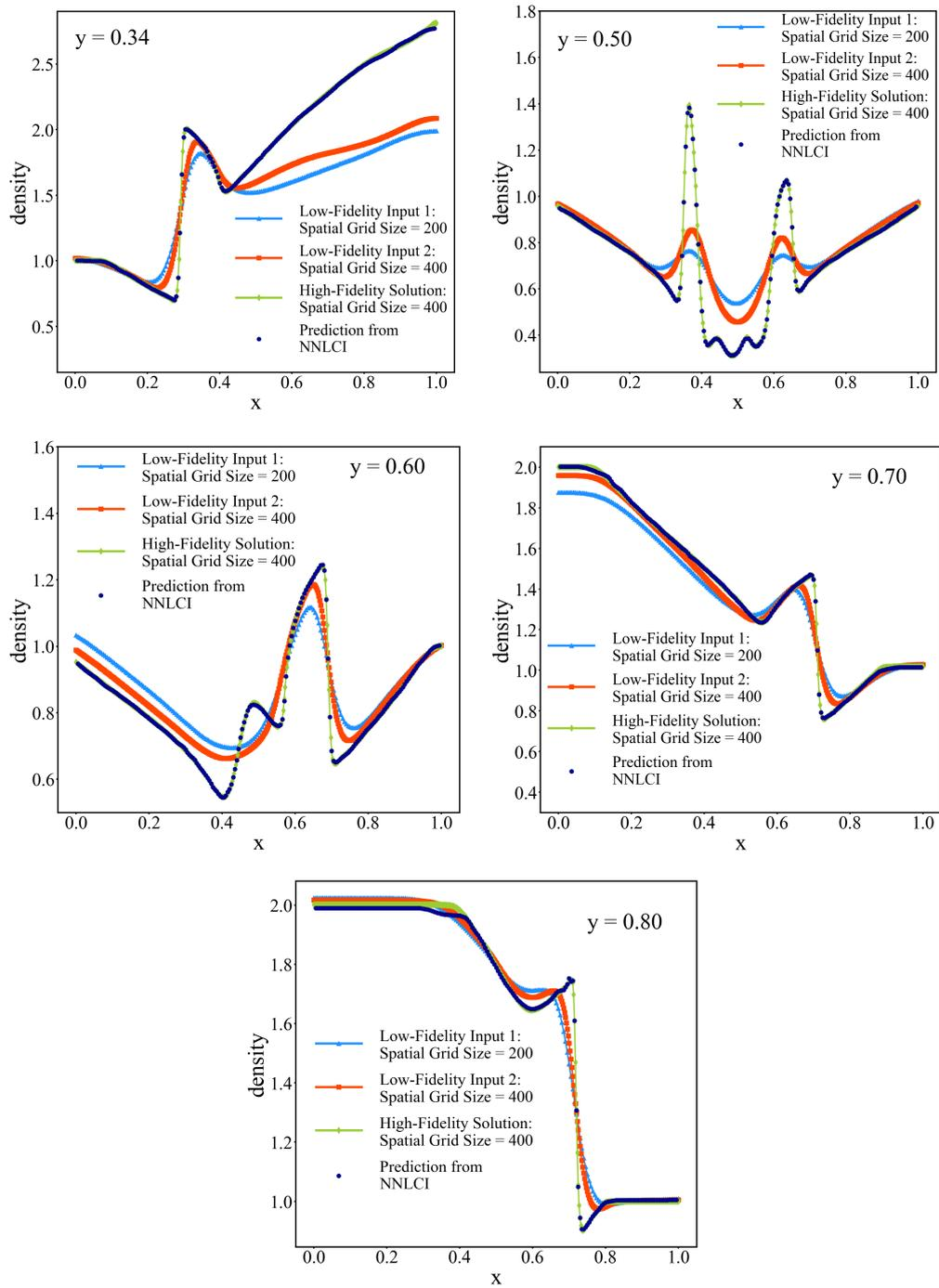
Figure 5: Axial distributions of density along  $y = 0.34$ ,  $y = 0.50$ ,  $y = 0.60$ ,  $y = 0.70$ , and  $y = 0.80$  of the NNLCI prediction of the final-time ( $t = 0.3$ ) solution of Case 6. Predicted density (dark blue), low-fidelity input solutions (blue and red) on  $200 \times 200$  and  $400 \times 400$  grids respectively, and reference solution (green).
