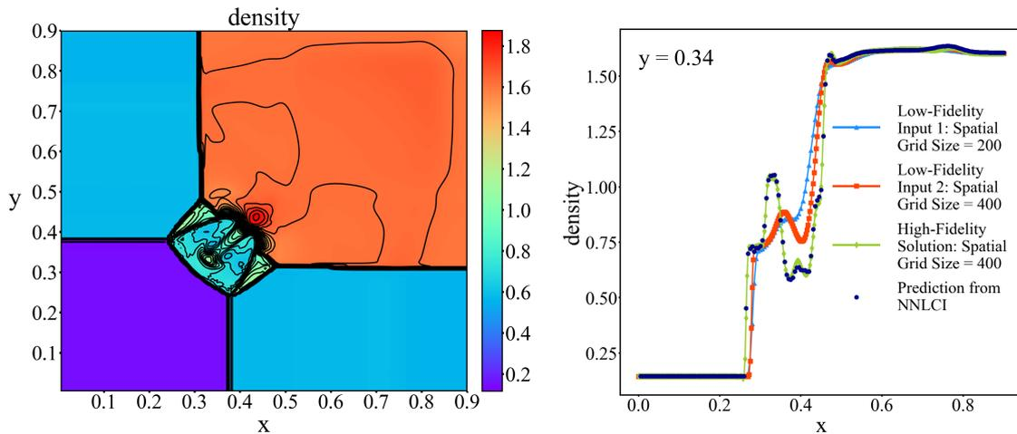
Figure 14: NNLCI prediction of final-time ( $t=0.3$ ) density distribution of 2D Euler system with initial value perturbed by +5% from that of Case 3 (see Table 1), and axial distribution of density (dark blue) along  $y=0.34$ , compared to low-fidelity input solutions (blue and red) on  $200 \times 200$  and  $400 \times 400$  grids, respectively, and reference solution (green).
