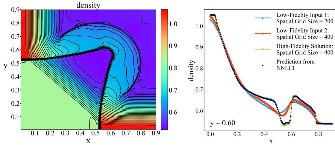
Figure 20: NNLCI prediction of final-time ( $t=0.25$ ) density distribution of 2D Euler system with initial value +5% perturbed from that of Case 8 (see Table 1), and axial distribution of density (dark blue) along  $y=0.60$ , compared to low-fidelity input solutions (blue and red) on  $200 \times 200$  and  $400 \times 400$  grids, respectively, and reference solution (green).
