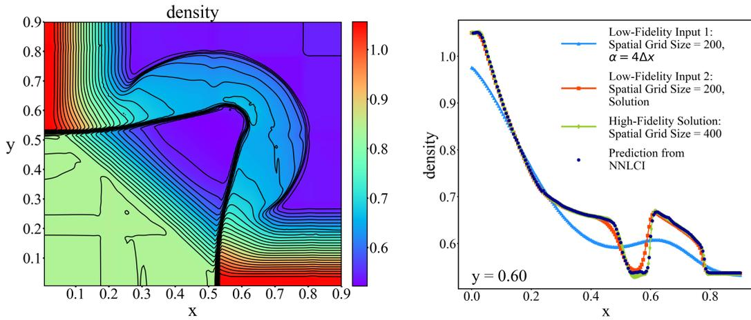
Figure 24: NNLCI prediction of final-time ( $t=0.25$ ) density distribution of 2D Euler system with initial value +5% perturbed from that of Case 8 (see Table 1), and axial distribution of density (dark blue) along  $y=0.60$ , compared to low-fidelity input solutions (blue and red) by leapfrog and diffusion splitting scheme (2.9) ( $\alpha=4\Delta x$ ) on  $400\times 400$  grid and 4th-order scheme on  $200\times 200$  grid, respectively, and reference solution (green).
