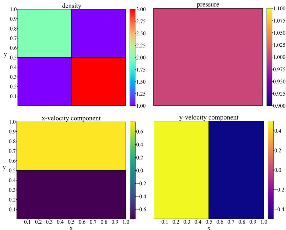
Figure 3: Initial values of Case 6: density, pressure,  $x$ -velocity, and  $y$ -velocity.
