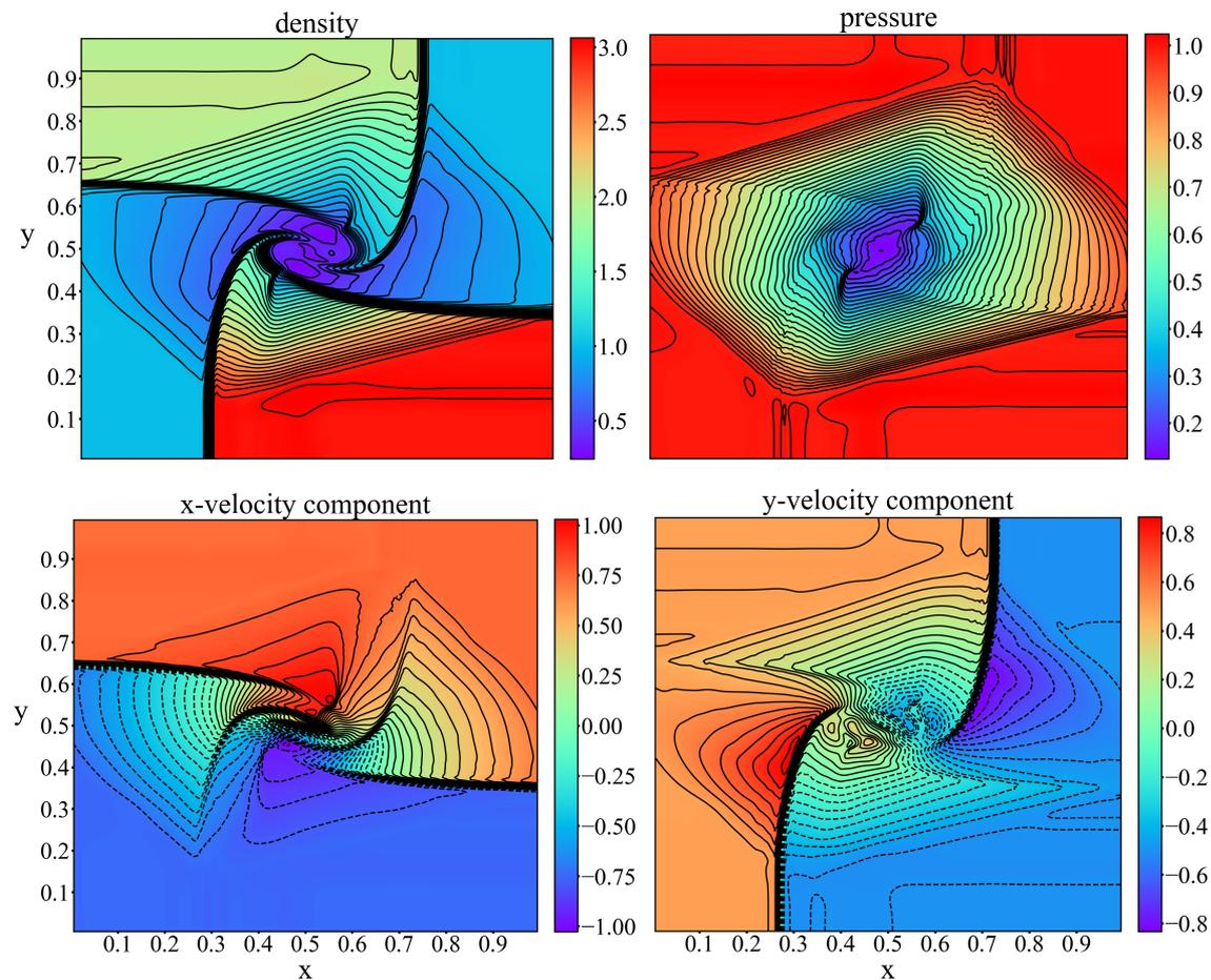
Figure 4: NNLCI prediction of the final-time ( $t=0.3$ ) solution of Case 6: density, pressure,  $x$ -velocity, and  $y$ -velocity.
