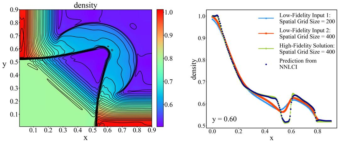
Figure 19: NNLCI prediction of final-time ( $t=0.25$ ) density distribution of Case 8 (see Table 1), and axial distribution of density (dark blue) along  $y=0.60$ , compared to low-fidelity input solutions (blue and red) on  $200 \times 200$  and  $400 \times 400$  grids, respectively, and reference solution (green).
