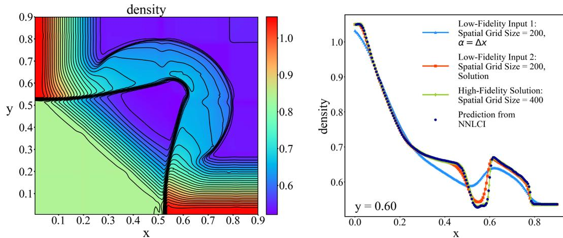
Figure 26: NNLCI prediction of final-time ( $t=0.25$ ) density distribution of 2D Euler system with initial value +5% perturbed from that of Case 8 (see Table 1), and axial distribution of density (dark blue) along  $y=0.60$ , compared to low-fidelity input solutions (blue and red) from leapfrog and diffusion splitting scheme (2.9) ( $\alpha=\Delta x$ ) on  $400 \times 400$  grid and 4th-order scheme on  $200 \times 200$  grid, respectively, and reference solution (green).
