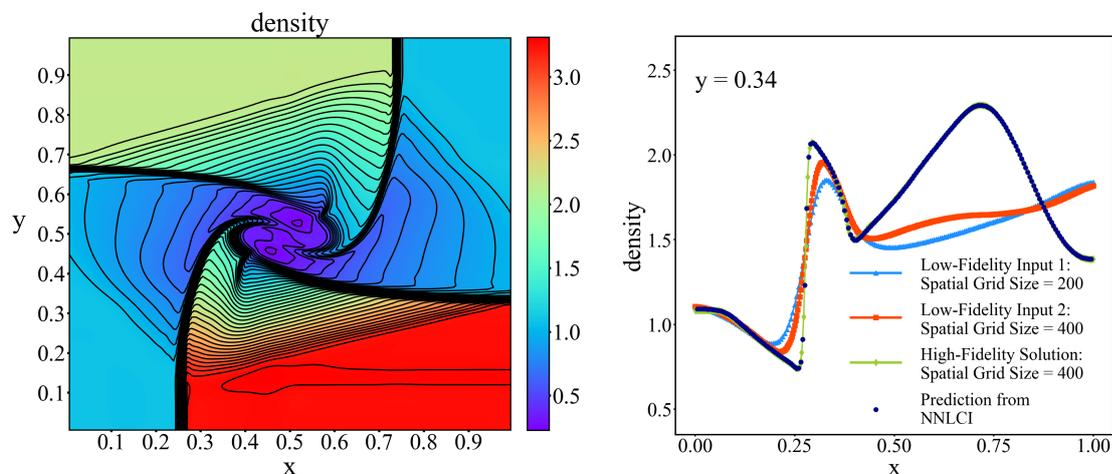
Figure 8: NNLCI prediction of final-time ( $t=0.3$ ) density distribution of 2D Euler system with initial value perturbed by +8% from that of Case 6 (see Table 1), and axial distribution of density (dark blue) along  $y=0.34$ , compared to low-fidelity input solutions (blue and red) on  $200 \times 200$  and  $400 \times 400$  grids, respectively, and reference solution (green).
