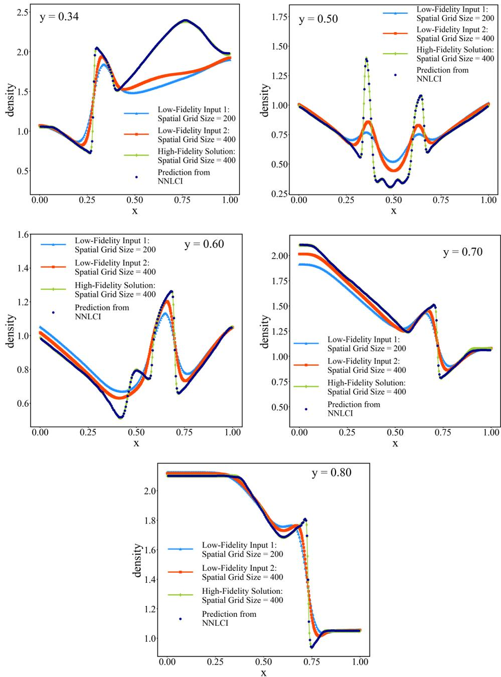
Figure 7: Axial distributions of density along  $y = 0.34$ ,  $y = 0.50$ ,  $y = 0.60$ ,  $y = 0.70$ , and  $y = 0.80$  of the NNLCI prediction of the final-time ( $t = 0.3$ ) solution of the 2D Euler system, with initial value +5% perturbed from that of Case 6. Predicted density (dark blue), low-fidelity input solutions (blue and red) on  $200 \times 200$  and  $400 \times 400$  grids respectively, and reference solution (green).
