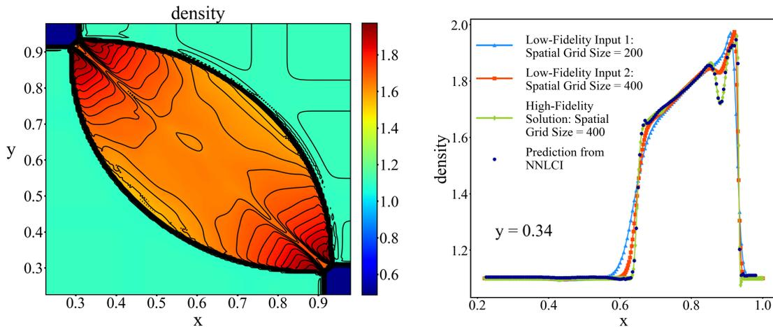
Figure 17: NNLCI prediction of final-time ( $t = 0.25$ ) density distribution of Case 4 (see Table 1), and axial distribution of density (dark blue) along  $y = 0.34$ , compared to low-fidelity input solutions (blue and red) on  $200 \times 200$  and  $400 \times 400$  grids, respectively, and reference solution (green).
