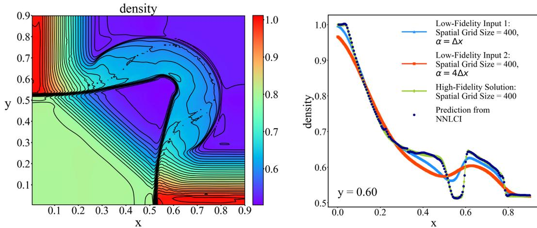
Figure 21: NNLCI prediction of final-time ( $t = 0.25$ ) density distribution of Case 8 (see Table 1), and axial distribution of density (dark blue) along  $y = 0.60$ , compared to low-fidelity input solutions (blue and red) from leapfrog and diffusion splitting schemes (3.1) and (3.2) ( $c = 4$ ), respectively on the  $400 \times 400$  grid, and reference solution (green).
