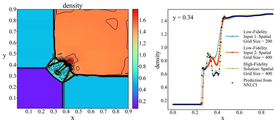
Figure 13: NNLCI prediction of final-time ( $t=0.3$ ) density distribution of Case 3 in (see Table 1), and axial distribution of density (dark blue) along  $y=0.34$ , compared to low-fidelity input solutions (blue and red) on  $200 \times 200$  and  $400 \times 400$  grids, respectively, and reference solution (green).
