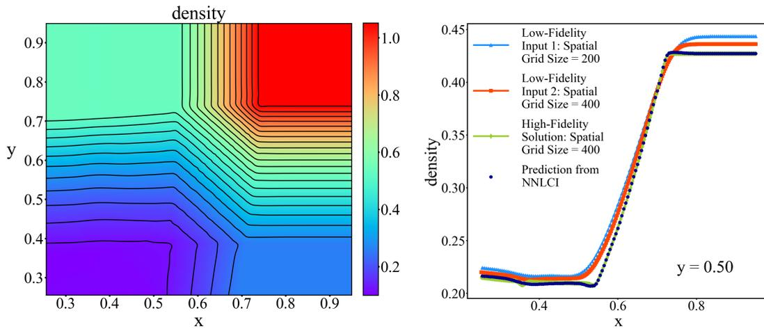
Figure 10: NNLCI prediction of final-time ( $t=0.2$ ) density distribution of 2D Euler system with initial value perturbed by +5% from that of Case 1 (see Table 1), and axial distribution of density (dark blue) along  $y=0.50$ , compared to low-fidelity input solutions (blue and red) on  $200 \times 200$  and  $400 \times 400$  grids, respectively, and reference solution (green).
