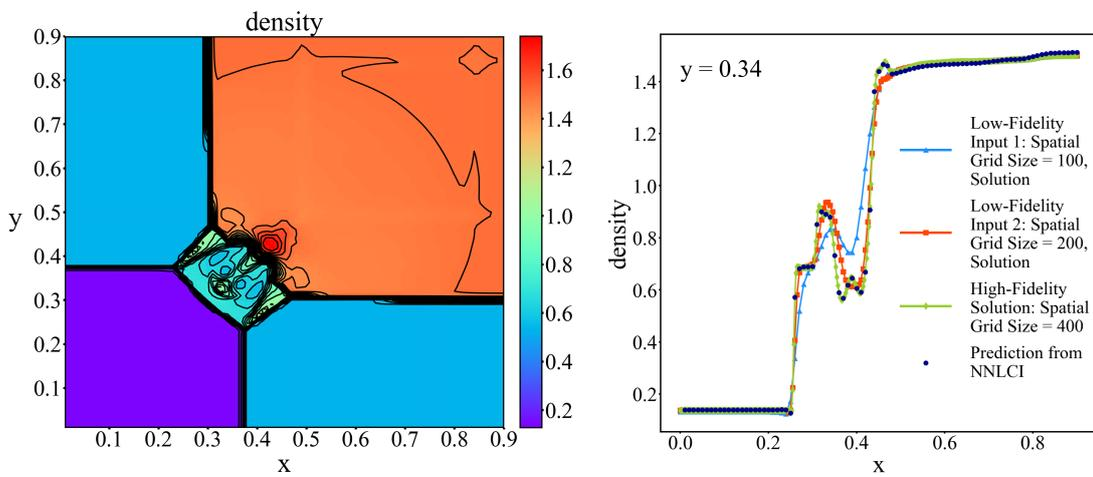
Figure 15: NNLCI prediction of final-time ( $t=0.3$ ) density distribution of Case 3 (see Table 1), and axial distribution of density (dark blue) along  $y=0.34$ , compared to low-fidelity input solutions (blue and red) on  $100 \times 100$  and  $200 \times 200$  grids, respectively, and reference solution (green).
