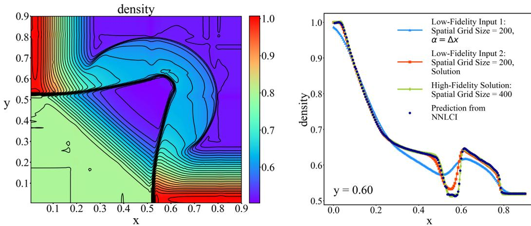
Figure 25: NNLCI prediction of final-time ( $t=0.25$ ) density distribution of Case 8 (see Table 1), and axial distribution of density (dark blue) along  $y=0.60$ , compared to low-fidelity input solutions (blue and red) from leapfrog and diffusion splitting scheme (2.9) ( $\alpha=\Delta x$ ) on  $400\times 400$  grid and 4th-order scheme on  $200\times 200$  grid, respectively, and reference solution (green).
