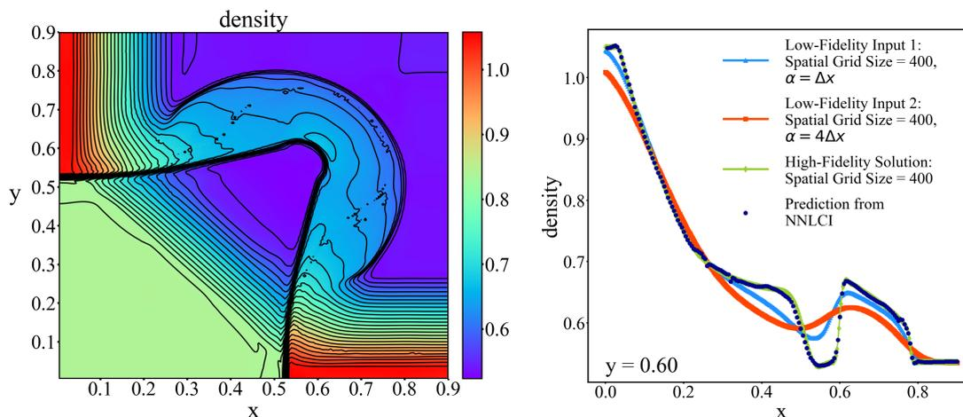
Figure 22: NNLCI prediction of final-time ( $t = 0.25$ ) density distribution of 2D Euler system with initial value +5% perturbed from that of Case 8 (see Table 1), and axial distribution of density (dark blue) along  $y = 0.60$ , compared to low-fidelity input solutions (blue and red) from leapfrog and diffusion splitting schemes (3.1) and (3.2) ( $c = 4$ ), respectively on the  $400 \times 400$  grid, and reference solution (green).
